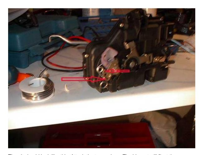
Then it should look like this. Attach the two springs. The biggest will fit at the upper arrow. The lower spring fits within the hole at the lower arrow and in the only little hole in the box (you'll see it).
