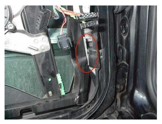
I took of the window mount, just because I got more room. Remember how it was mounted.. Would be easier to remount. The prev pic showed 4 green rings. Torx 45. When remounting, you should fasten the upper two before the torx on the bottom (work right to left)
