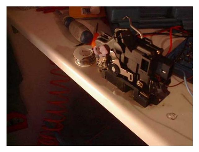
You'll have to wiggle a a bit to get this arm right, and I had to set the torx screw just inside, so I could pull out the white rod that the metallic/plastic arms are connected to. You'll figure it out! Don't screw tight before you see that the white rod are lined up with the white arm.
