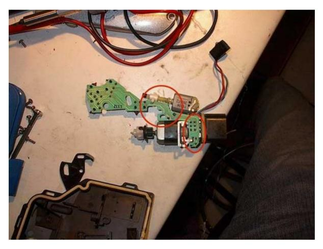
Here's the circuit board. The rings shows where most of the corrosion where. On the thin electric lines and down by the connector (on the other side - se pic below).
