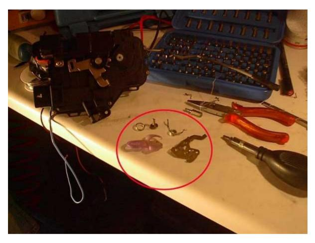
The four parts left after you've put the two main parts together (all the torx) You'll then have 4 remaining parts - 2 springs, one plastic and one metal arm. (and one screw of course).
