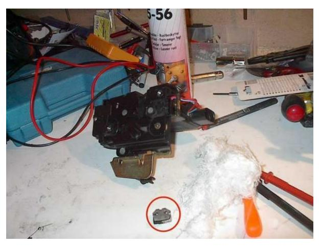
The red ring shows the metallic clamp that holds the sensor to the latch. Just flips off.
