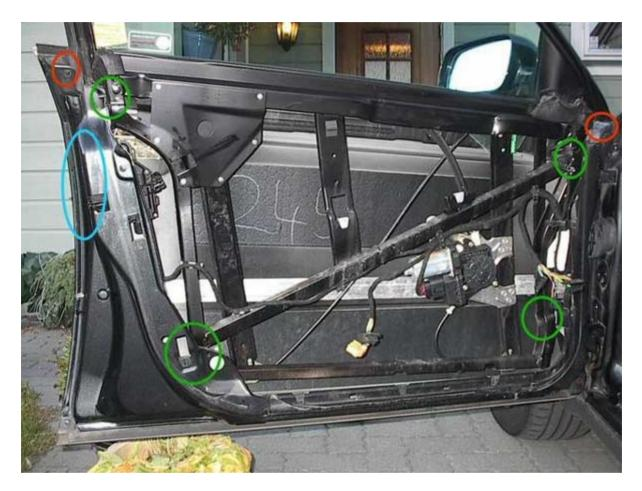
The blue rings shows two M8 screws that actually holds the latch. Flip off the plastic that hold the lock rod. Pull that rod off. Then the key rod. You'll have to wiggle that out (pull a bit down and turn clockwise, it just holds by the rods length).
