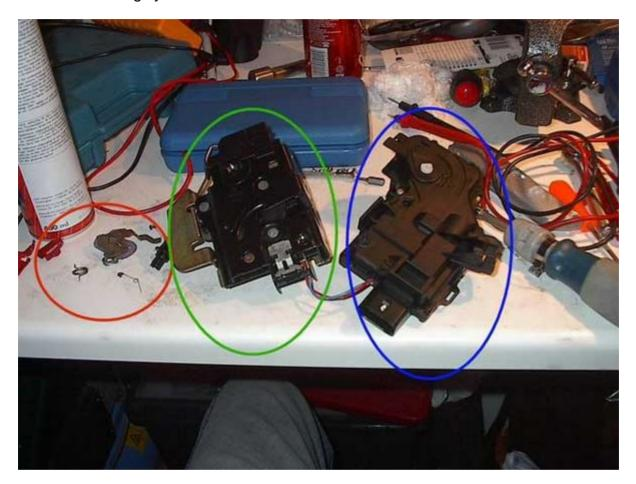
This was a tricky job, first off I saw 2 springs connecting the locking mechanism. Split the two parts (2 torx-20 + 1 torx-10 and two plastic locks) and open the box containing the circuit board (6-7 torx-10).
