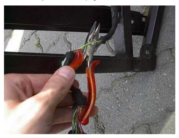
Reattach the latch and hot-wire the new connectors you made into the wires from the car. For my experience, I had to make new connectors for line 4 and 6.
