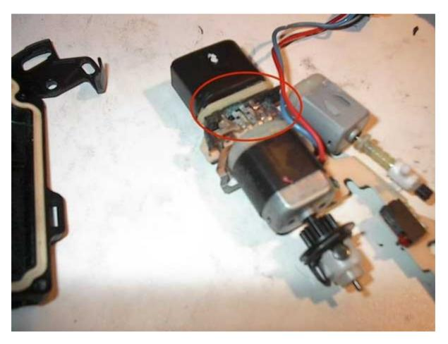
Ugh.. bad pic, but you see the corrosion. When the latch is installed, this is the absolute bottom of the box - and when the box is not tight, water/damp concentrates here..
