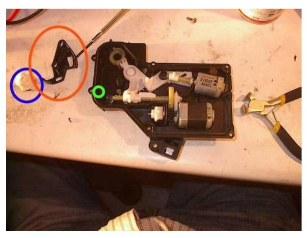
The orange ring around plastic arm has to be refitted when the circuit board is in place. The "arm" of this, will touch the micro switches on the downside - left of the circuit board. The micro switch I'm talking about is about where the green ring is, when you've reattached the circuit board.
